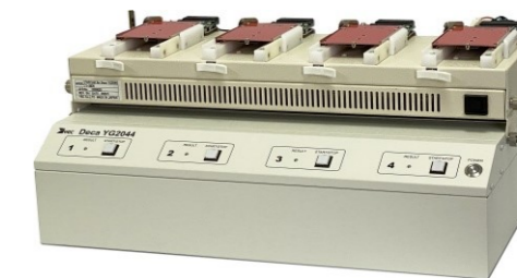
U.2 NVMe Quick Loader Plug-in Jig Attached
