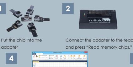
Rearrange the physical NAND blocks into the logical block by using VNR software
